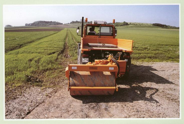
This is the unique machine for road building and maintenance and for landscaping. The high impact-force makes a very good job of compacting.
